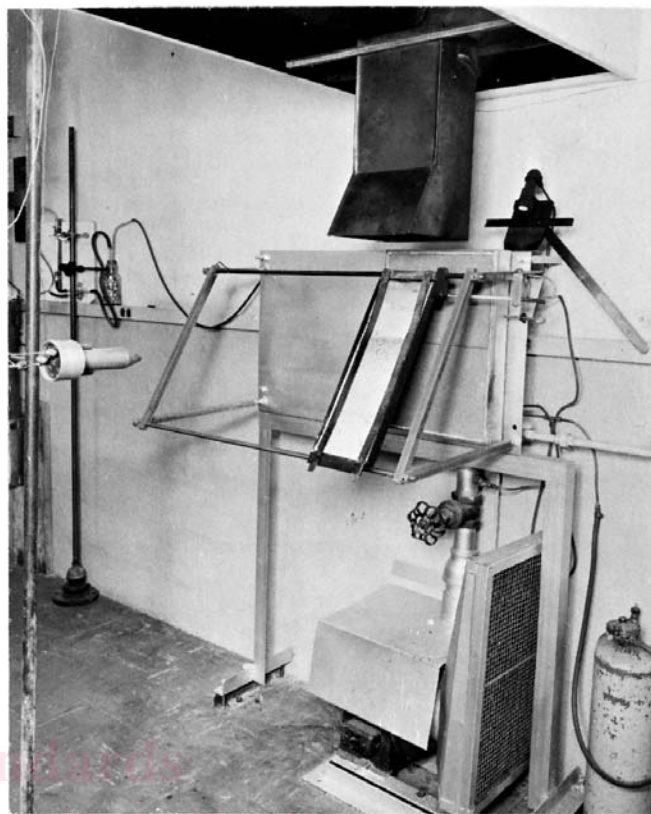
FIG. 1 Radiant Panel Flame Spread Test Equipment
