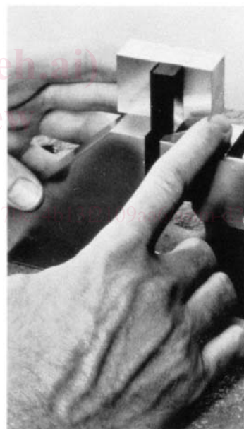
FIG. 4 Jig for Positioning Specimen for Clamping
