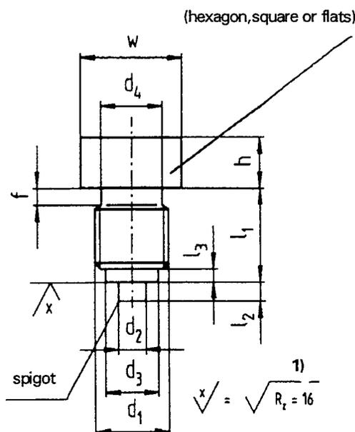
NOTE : Minimum height  $h$  of flats shall be compatible with use of standard spanners according to ISO 10102.
