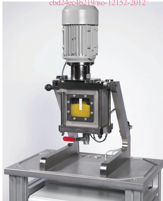
Figure 2 — Overall view of a foam tester
