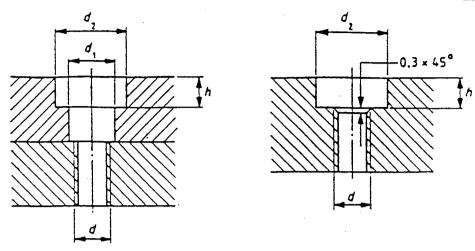
The values of the dimensions of protective shrouds and counterbores in the alternative arrangements shown are listed in Table 1.
