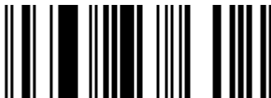
Figure 1 — GS1 DataBar Omnidirectional symbol representing (01)20012345678909
