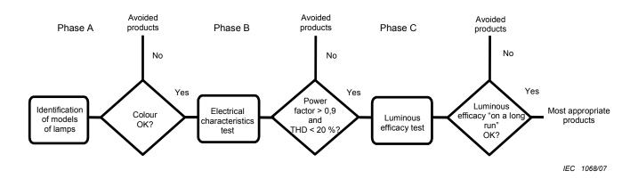
Figure 1 – Lamps selection test programme
