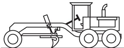
**Figure 2 — Six-wheel grader**
