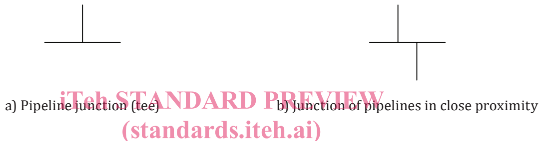
Figure 6 — Representation of connected pipes
