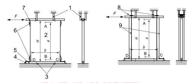
a) Example with end restraints PRF b) Example with tie-down rods
