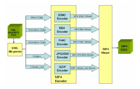
Figure AMD22.1 — MP4XMLEncoder structure
