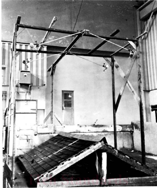
( https://standards.iteh.ai ) FIG. 3 Rain Test Apparatus
