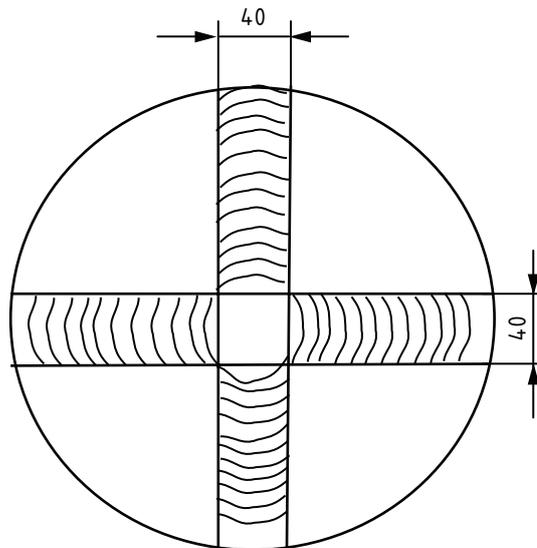
Figure 2 — General cutting pattern of heart planks from a log of diameter  $\leq 180$  mm
