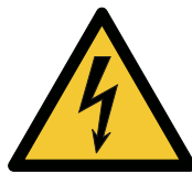
Figure 1 — Symbol of voltage class B electric components
