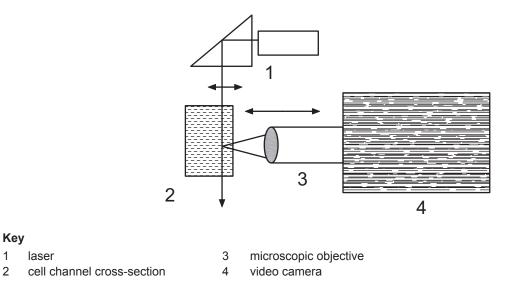
Figure 2 — A typical electrophoresis video microscope
