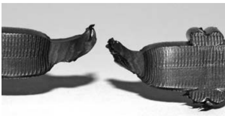
FIG. 2 Ductile Rupture Outside Fusion Interface
