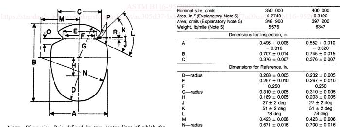
NOTE—Dimension R is defined by two center lines of which the upper is the center line of the radius of the groove, and the lower is the center line of the groove.
