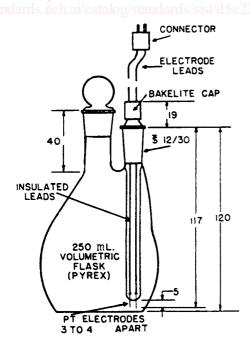
Note 1—All dimensions in millimetres. FIG. 1 Titration Flask Assembly
