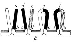
ad = cut pile tuft element gj = loop pile tuft element ab, cd, ef, gh, ij, jk = tuft legs cd, ef = cut pile tuft leg pair ij, jk = loop pile tuft leg pair, a loop B = one binding site
