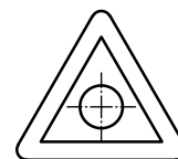
c) TN.G with chip breakers on both faces
