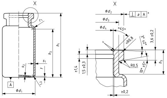
а The perpendicularity tolerance a (as defined in ISO 1101) is a limit for the deviation of the plumb-line through the centre of the bottom part and the axis of the vial at the upper edge of the flange; it is measured at the brim.
