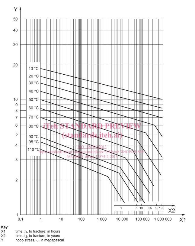
Figure 2 — Reference curves for expected strength of PP-B
