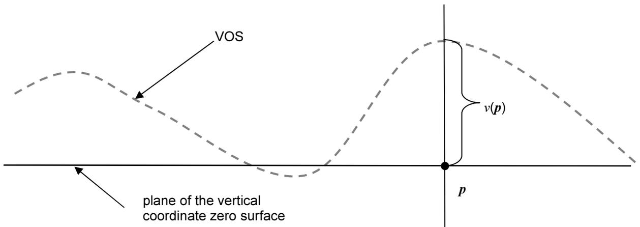
Figure 9.2 — Vertical offset surface tangent plane
