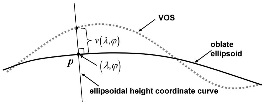
Figure 9.1 — Vertical offset surface for ellipsoidal height
