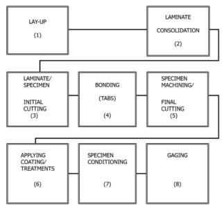
Note 1—Material identification is mandatory. Continuous traceability of specimens is required throughout the process.
