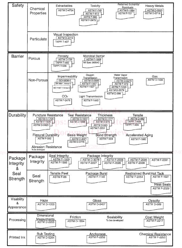
FIG. 1 Summary of Test Methods for Medical Packaging Design and Evaluation
