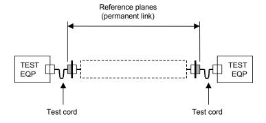
NOTE The dotted area contains cable and may contain splices and additional connections.
