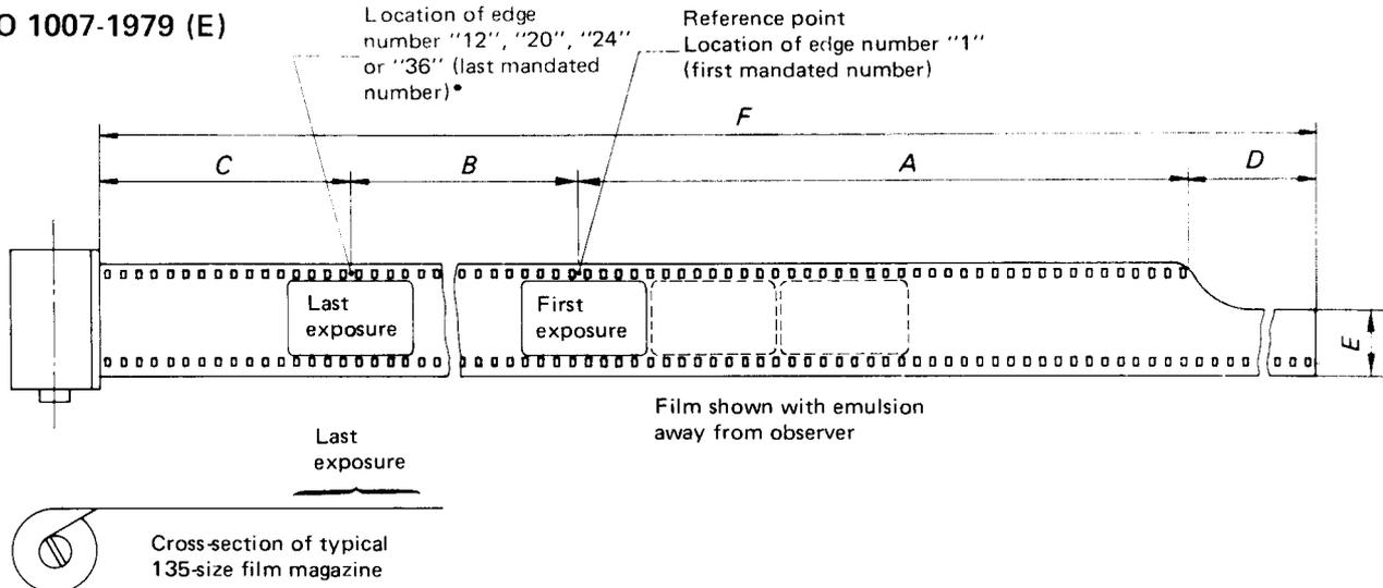
• The edge numbers, 12, 20, 24 and 36 may be replaced by their equivalents 23, 39, 47 and 71 of the permissible half-frame series.
