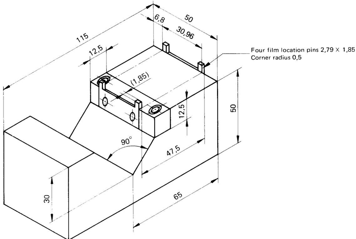
FIGURE 6 – Gauging jig for measurement of film magazine dimensions relative to edge of film in 135-size film magazine
