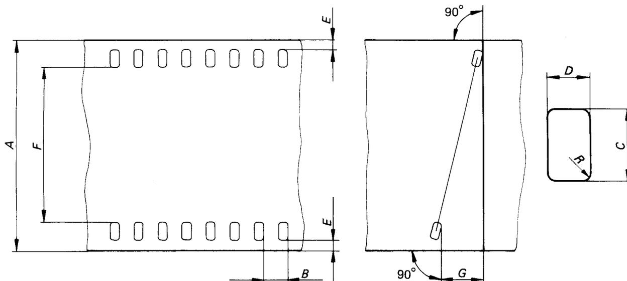
FIGURE 2 — Perforating dimensions for 135-size film
