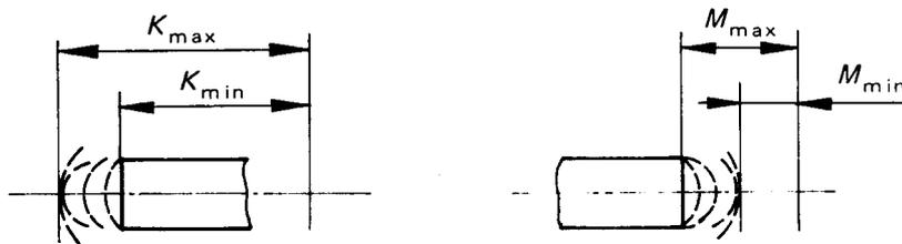
FIGURE 4 – Rounded spool splines
