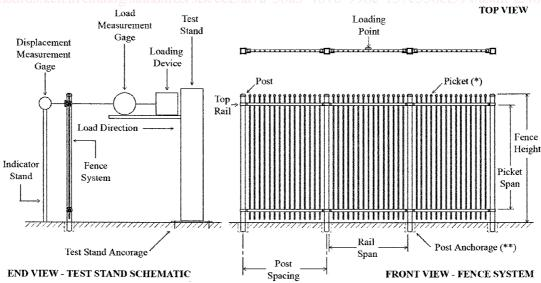
Note 1 - Any picket point style is acceptable on tested system; pickets may extend through the rails (as shown) or may terminate at
