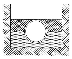
Note 1—Pipe is bedded to its centerline in compacted granular material with a minimum of 4 in. (102 mm) under the pipe. Compacted granular or select<sup>A</sup> material is used to the top of the pipe. (Material is compacted to approximately 90 % Standard Proctor in accordance with AASHTO Standard T-99.)
