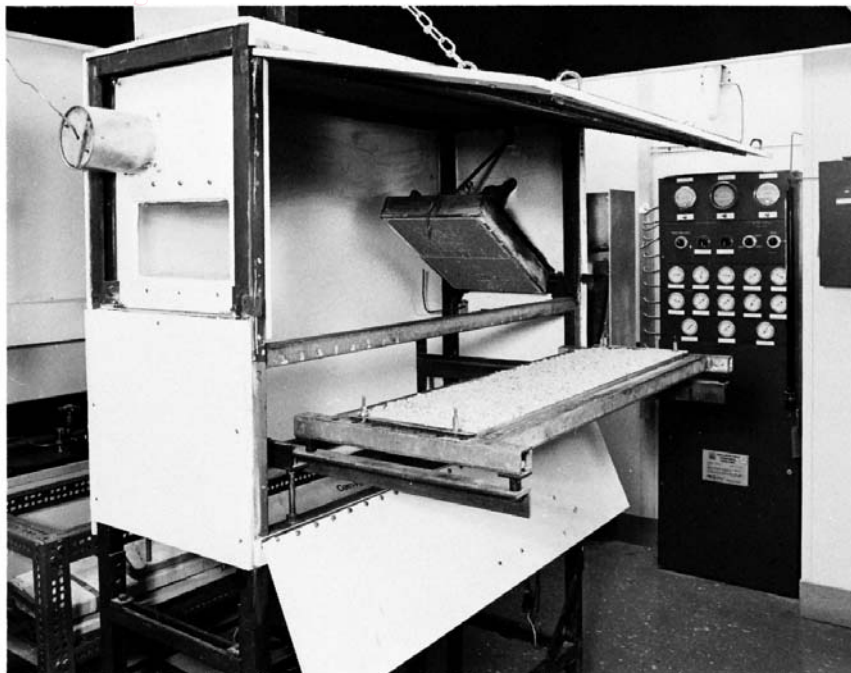
FIG. 1 Radiant Test Panel Chamber
