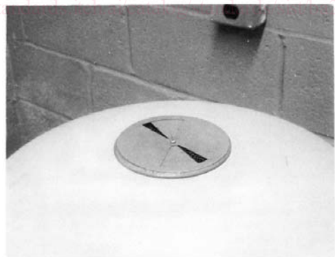
FIG. 2 Choking Air Inlet of Chamber (Sorvall Centrifuge)
