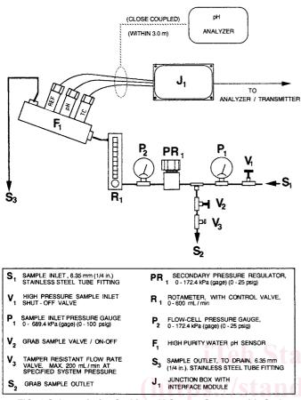
FIG. 1 Schematic for On-Line pH Sensor System with Grab Sample Outlet
