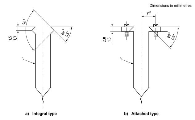
Knife edges shall be square with specimen surfaces and parallel to  $\pm 0.5^{\circ}$ .
