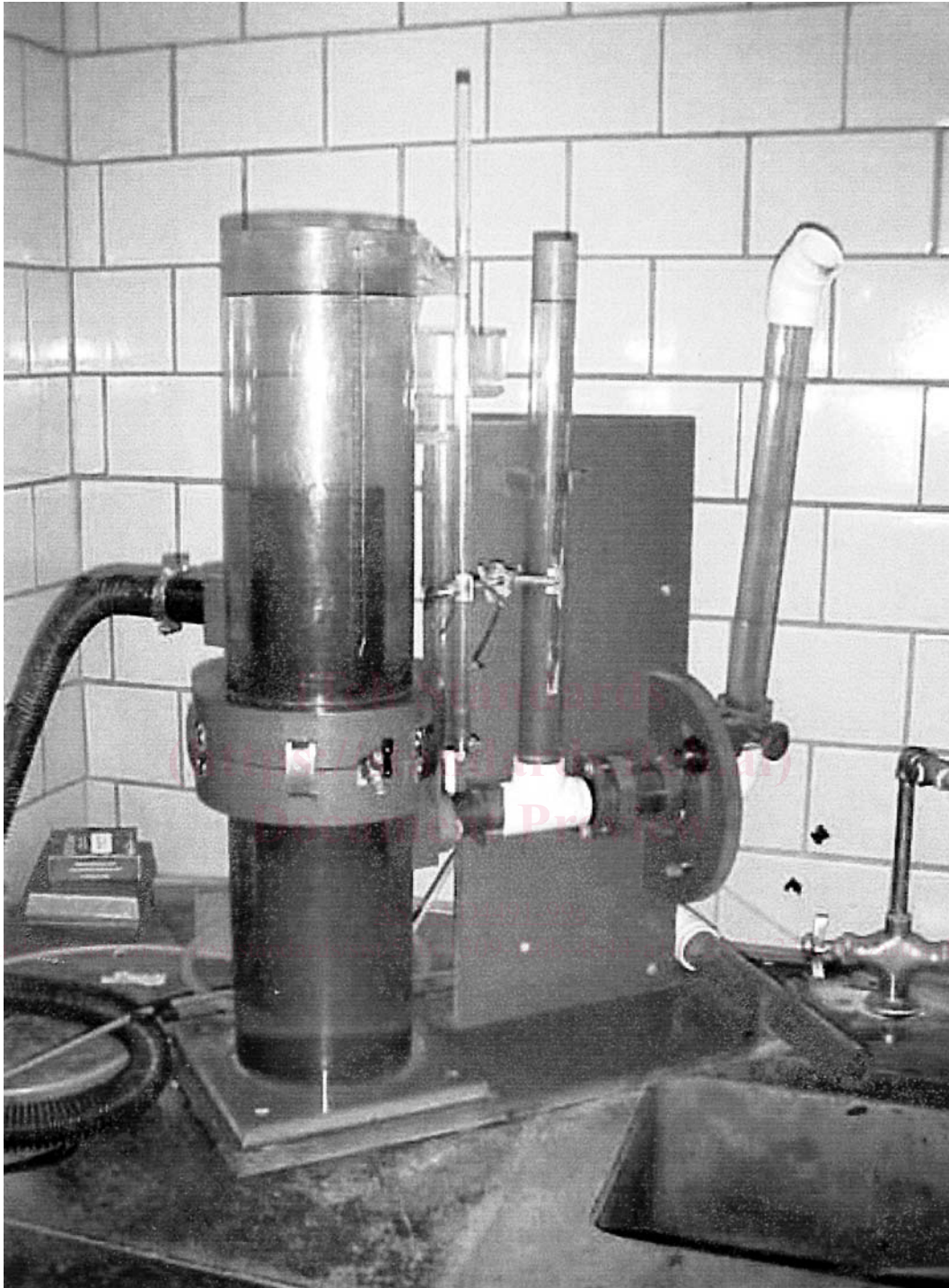
FIG. 1 Constant and Falling Head Permeability Apparatus
