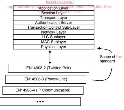
Figure 1 — Relationship of CNP 3 specification to CNP 1 specification
