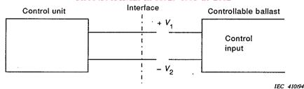
The lamp power (light output) of a controllable ballast is controlled by the d.c. voltage on the control input of the controllable ballast. The d.c. voltage has the following characteristics:
