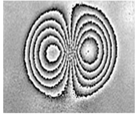
FIG. 3 A phase map shearogram with horizontal shear vector yields a fringe pattern showing the first derivative of the out-of-plane deformation, \partial w / \partial x . Using an unwrapping algorithm, the image at right shows the positive (white) and negative (black) slope change.
