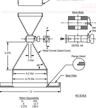
6.75 12 FIG. 1 Density Apparatus
