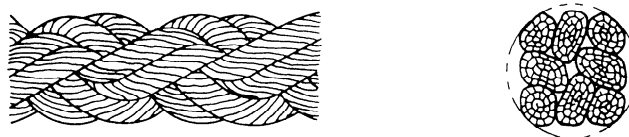
Figure 2 — Shape of an 8-strand plaited rope (type E)
