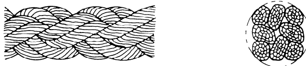
Figure 2 — Shape of an 8-strand plaited rope (type E)
