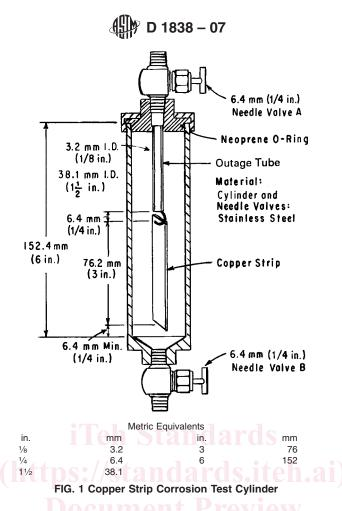
5.1.2 The assembly shall be verified for gas tightness by leak testing at 3450 kPa (500 psig) with inert gas prior to first use, whenever pressure-containing components of the assembly are replaced, or otherwise on an annual basis.
