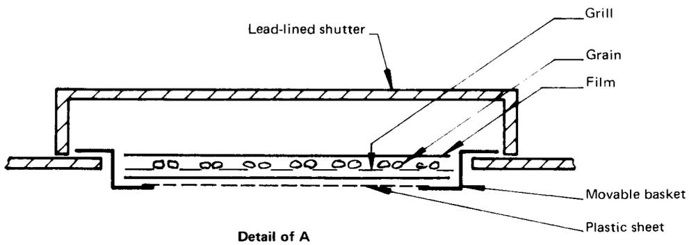
FIGURE 2 – Diagram of another form of assembly of X-ray apparatus
