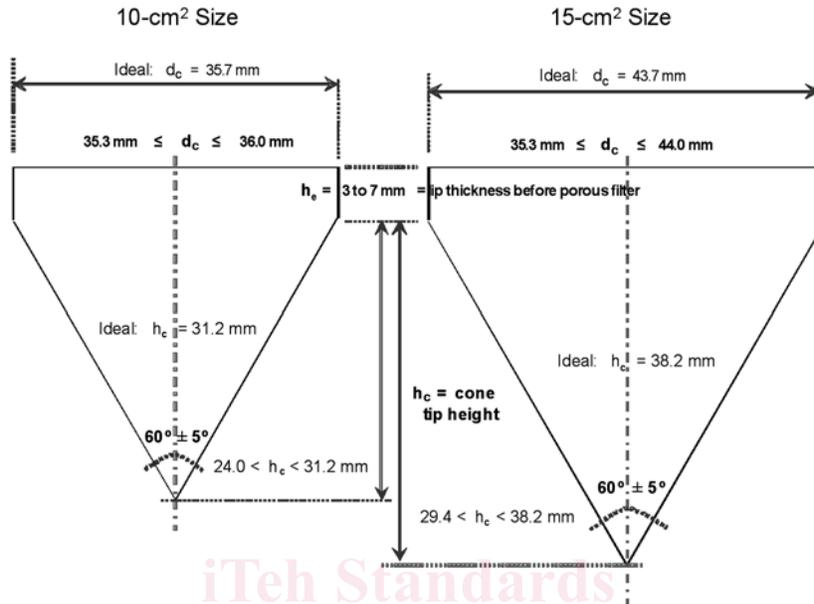
FIG. 2 Manufacturing and Operating Tolerances of Cones (3)
