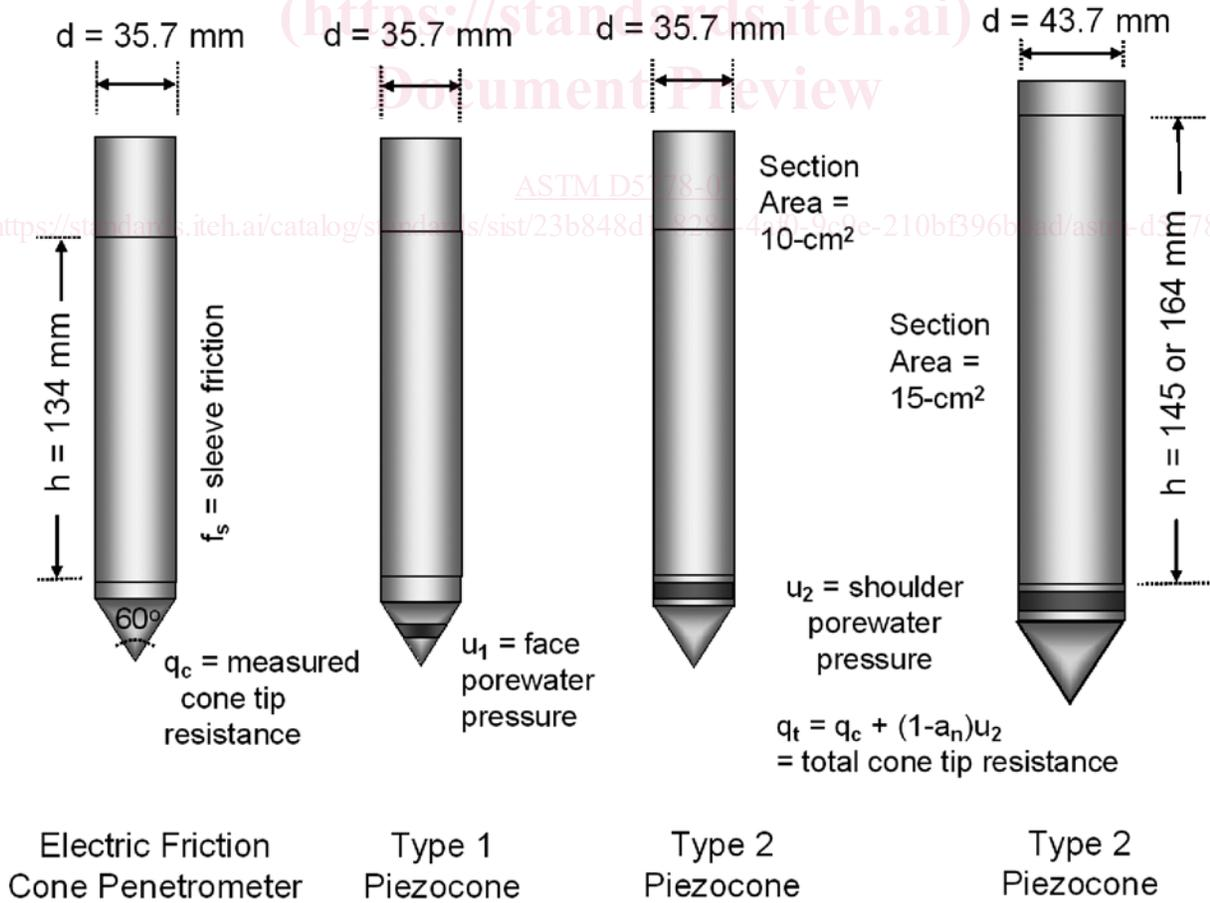
FIG. 3 Penitrometer Design Configurations: (a) Electronic Friction-type, (b) Type 1 Piezocone, (c) Standard 10-cm<sup>2</sup> Type 2 Piezocone, and (d) 15-cm<sup>2</sup> Type 2 Version (5)
