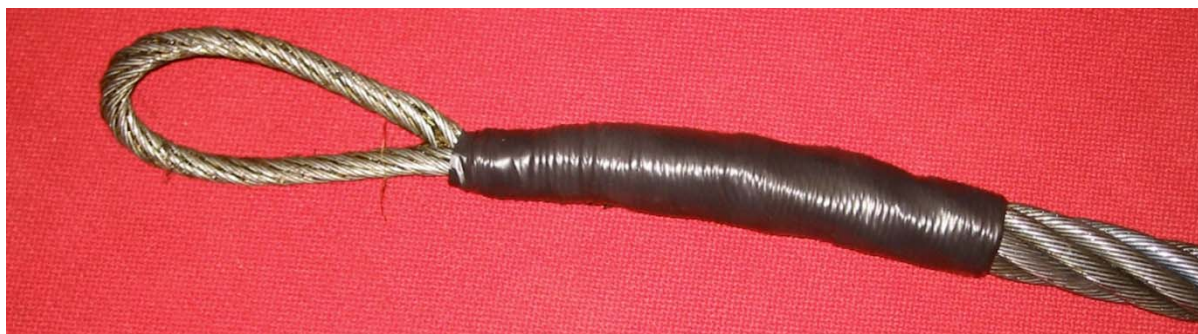
Figure 2 Completed flexible pulling eye made from the steel core itself
