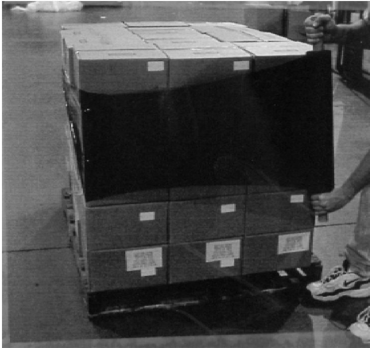
FIG. 4 Extended Core Hand Film (as defined in 16.2.1)
