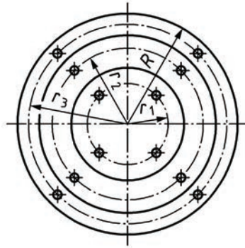
Figure 2 — Air velocity measuring points of round duct
