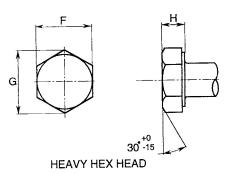
DIMENSIONS FOR TWIST OFF STRUCTURAL BOLT
