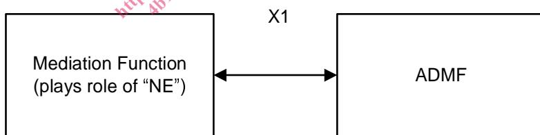
**Figure 4: X1 deployment model for Mediation Functions**
