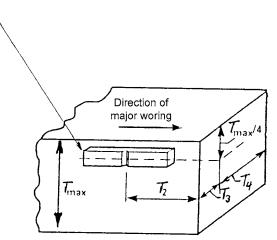
Note 1—For material with thickness *T* greater than 2 in. [50 mm],  $T_2=T_3=T_4 \ge T_{\text{max}}$ where:  $T_{\text{max}}$ = maximum heat treated thickness
