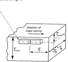
NOTE 1—For material with thickness *T* greater than 2 in. [50 mm],  $T_2=T_3=T_4\geq T_{max}$ where:
